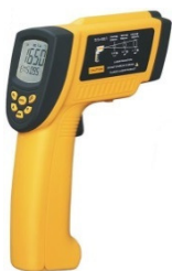
Figure 17. A typical infra-red thermometer, suitable for measuring heating of a crop canopy due to reduced evaporative cooling associated with crop water stress.
