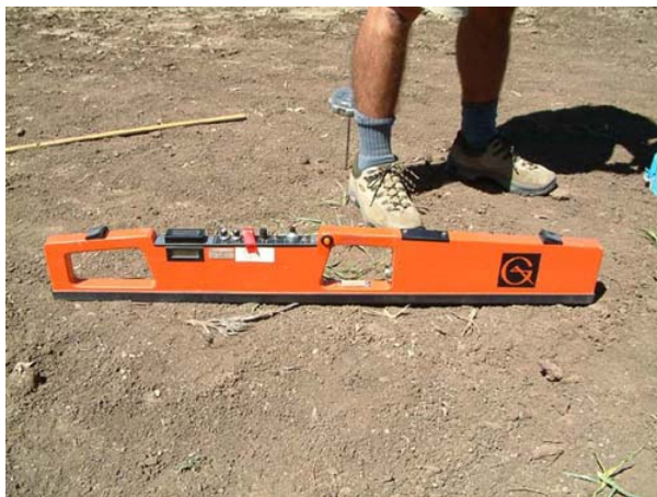
Figure 12. An EM38 being used in vertical mode. The coils are located at each end of the device. Image from ( http://www.usyd.edu.au/agric/web04/Group%201%20Web%20page/EM38%20Final.htm )
